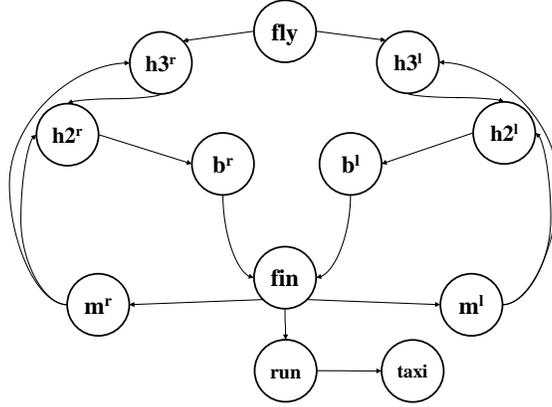
Figure 3.2: SATS locations, transitions, and invariants for aircraft  $i$ . The continuous variable  $x[i]$  only matters in states  $\mathbf{b}^r$ ,  $\mathbf{b}^l$ ,  $\mathbf{fin}$ ,  $\mathbf{m}^r$ , and  $\mathbf{m}^l$ , which correspond to when  $i$  is attempting to land on the runway by reaching location  $\mathbf{run}$ . Invariants for continuous variables in locations are captured by, for instance,  $x[i] \leq L_B$ , etc., for some  $L_B > 0$ .
