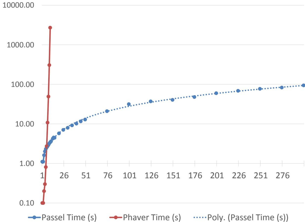
Figure 7.4: Anonymized reachability runtime comparison of PHAVer and *Passel* for MUX-SEM. The vertical axis scale is logarithmic. The horizontal axis is the number of automata  $N$ . This illustrates scaling to hundreds of automata.
