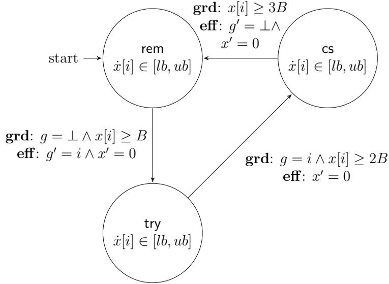
Figure 4.12: MUX-INDEX-RECT mutual exclusion algorithm of Figure 4.11.
