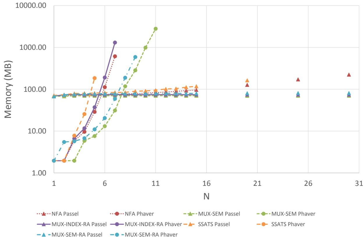
Figure 7.3: Anonymized reachability memory usage comparison of PHAVer and *Passel* for several examples. The vertical axis scale is logarithmic and has units of megabytes. The horizontal axis is the number of automata  $N$ .
