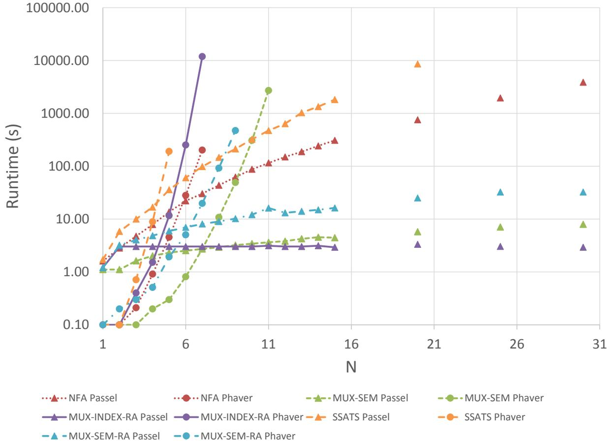
Figure 7.2: Anonymized reachability runtime comparison of PHAVer and *Passel* for several examples. The vertical axis is logarithmic and has units of seconds. The horizontal axis is the number of automata  $N$ .
