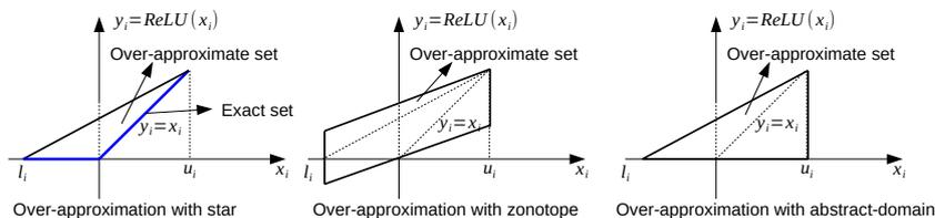
Fig. 2: Over-approximation of ReLU functions with different approaches.
