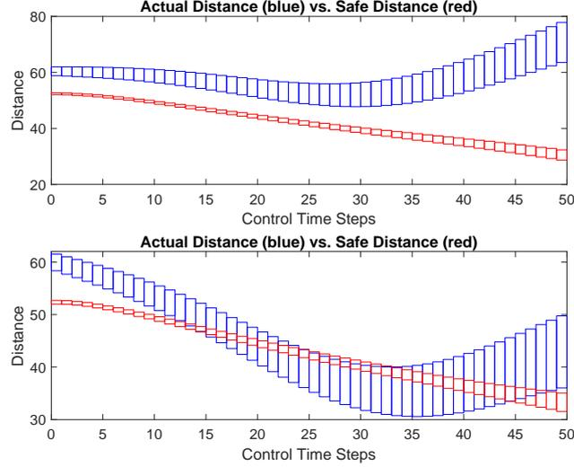
Fig. 3: Two scenarios of the ACC system. In the first (top) scenario ( $v_{lead}(0) \in [29, 30]m/s$ ), safety is guaranteed,  $D_{rel} \geq D_{safe}$ . In the second scenario (bottom) ( $v_{lead}(0) \in [24, 25]m/s$ ), safety is violated since  $D_{ref} < D_{safe}$  in some control steps.
