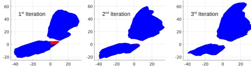
Fig. 6: The evolution of the output reachable domain on Property 1&2 in the repair of Agent 1 on ID 1. The domain is projected on  $(y_2, y_3)$ . The blue area represents the exact output reachable domain while the red area represents the unsafe reachable domain.
