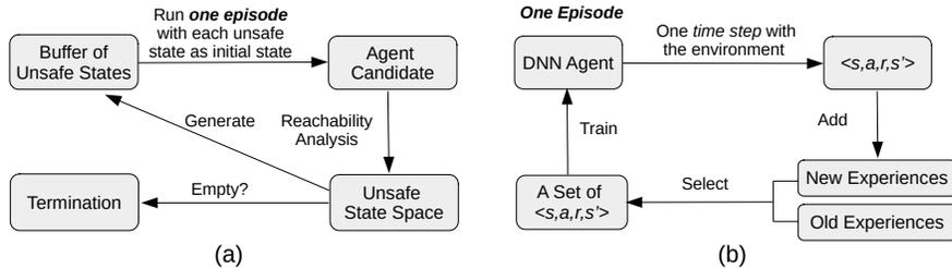
Fig. 2: Repair framework for deep reinforcement learning. In the loop (a), given an agent, its unsafe state space is first computed with our reachability analysis method. Then, *episodes* in (b) are run with unsafe states as initial states to update the agent, where the occurrence of unsafe states will be penalized.
