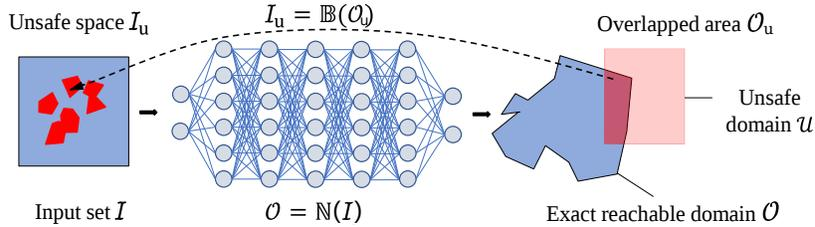
Fig. 1: Computation of the unsafe input-output reachable domain  $\mathcal{I}_u \times \mathcal{O}_u$ .
